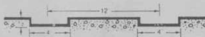
Grooves are 4" wide x 1/2" deep on 12" centers Metric — (100.8mm x 12.70mm on 304.8mm centers)
