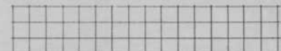
Grooves are 1/2" wide x 1/4" deep on 2" centers Metric — (6.35mm x 6.35mm on 50.4mm centers)
